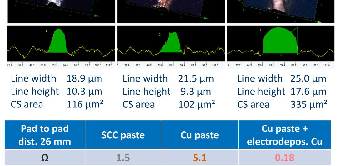
paste copper is alone very high. The efficiency of cells having lines of only printed copper is at 6% ! With additionally electrodeposited copper 22.3% are achieved.
