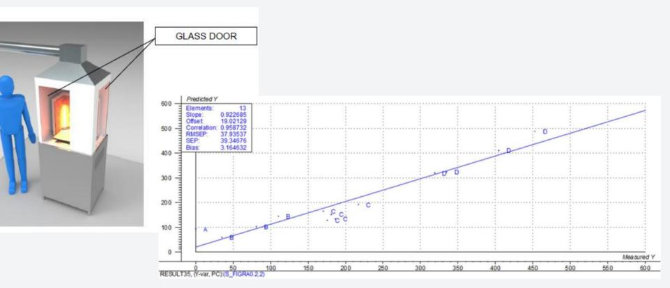
A statistical analysis has been used to establish an empirical correlation between the MINI-SBI and the standard SBI results
