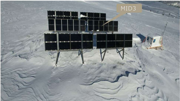
Position of device under test (DUT), Solitek SOLID Alpin prototype 560Wp (since 11/2023)
