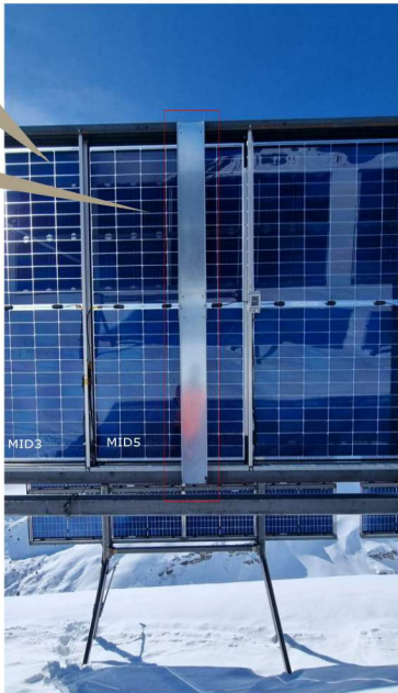
Shading mock-up on module back side at test facility Tschers (144HC Alpin, portrait) azimuth 0° S, inclination: 65° (OTF22) Source: ewz, ZENDRA, Gantner Instruments
