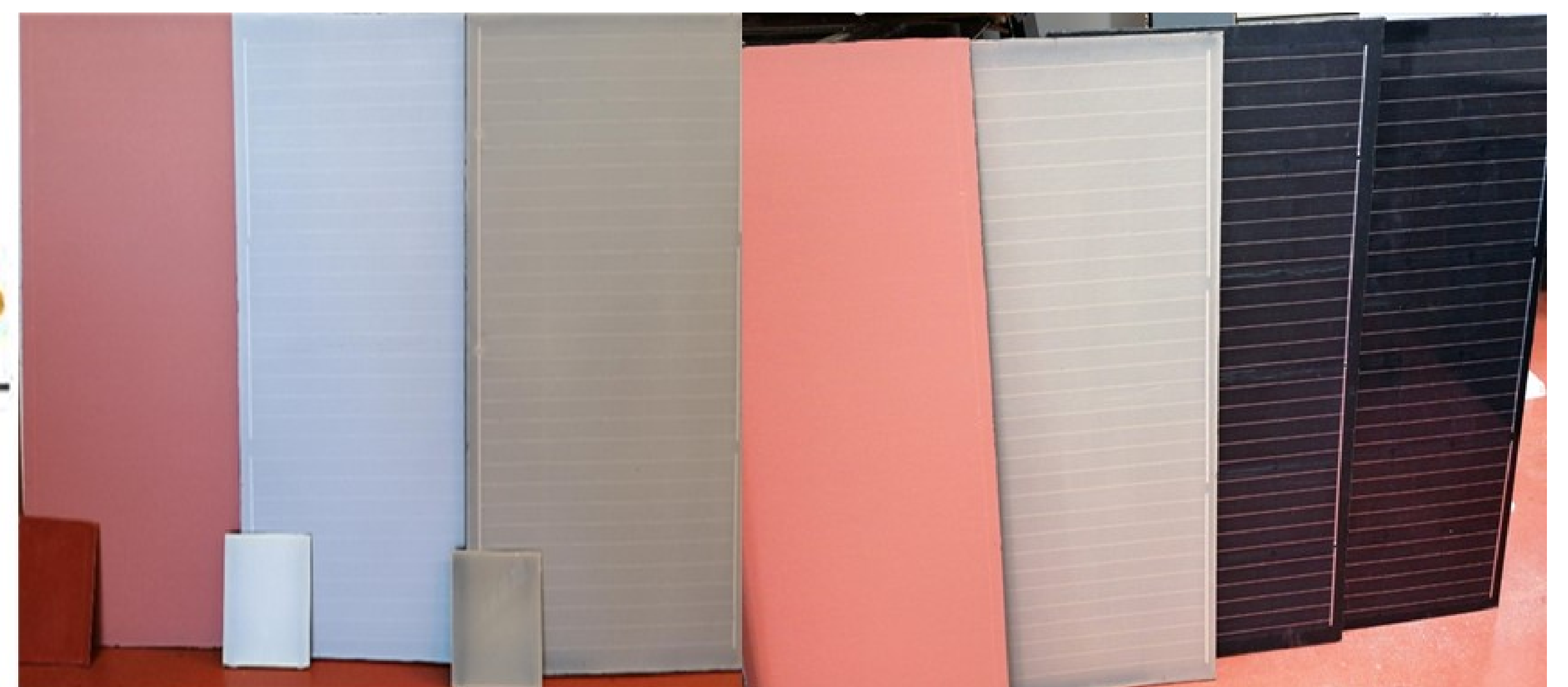
Figure 3: photo of colored (0.1x1) m2 LW PV modules and the respective mini-modules at the bottom
