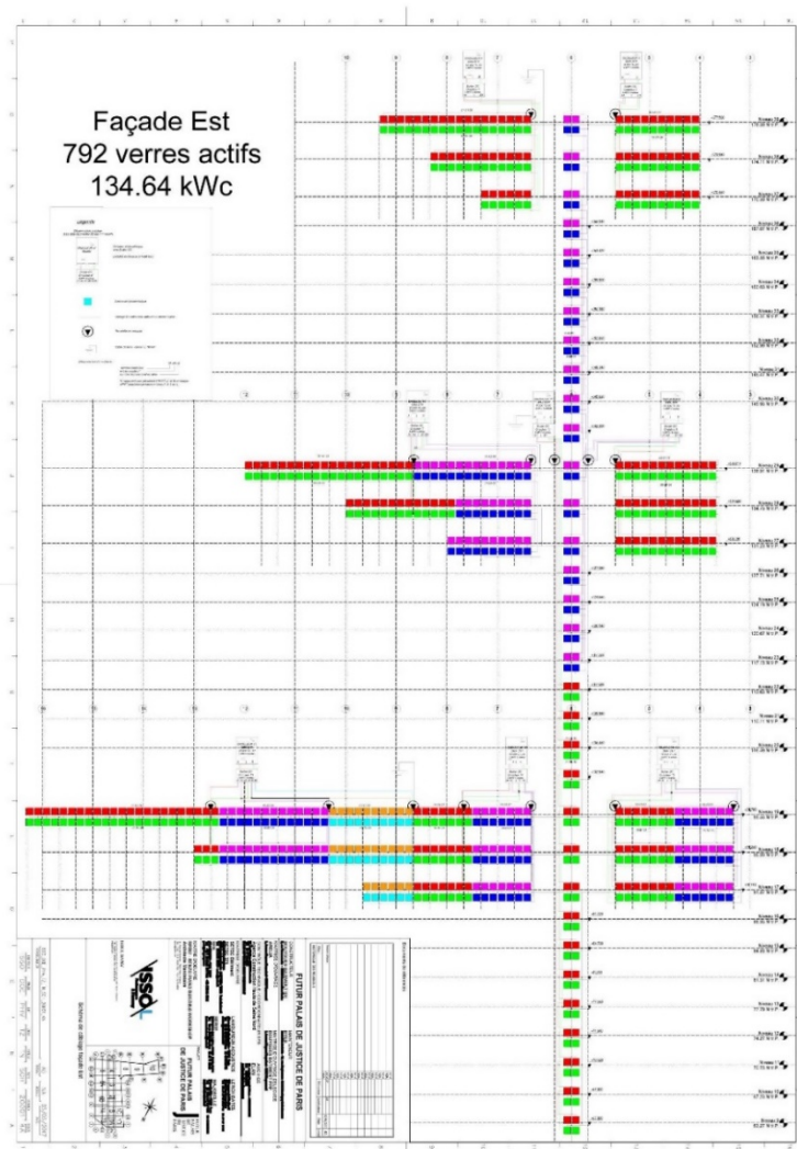
as built drawing of the east elevation showing the typology of cabling
