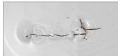
High intensity hot spots in PVDF-based backsheets
