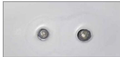
Bubbling leads to cracking
