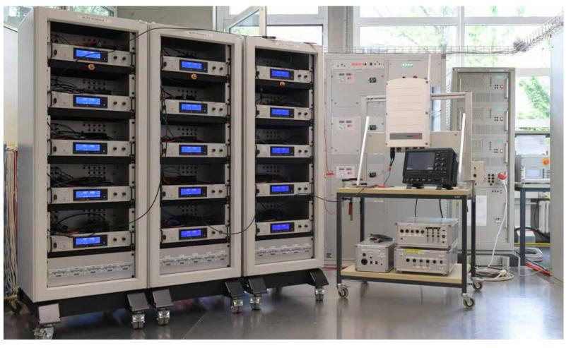
Grid connection, inverter and power electronics testing.
